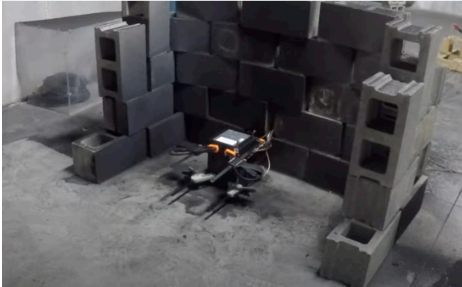
Figure A.2. (a) Stack of fully-charged pouch cells in fire bunker for thermal runaway tests. (b) The first cell fails explosively in a white-hot fireball at 0:09/2:13 minutes. Subsequent jets of flame last another 8 seconds; a second cell goes into thermal runaway (0:33/2:13 minutes) with a similar fireball, lasting about 5 seconds; and 5 or 6 such fireballs occur up to 1:55/2:13 mins of the recording.
