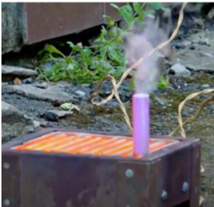
Figure A.1: (a) A charged 2.6 Ah cell being deliberately overheated.
