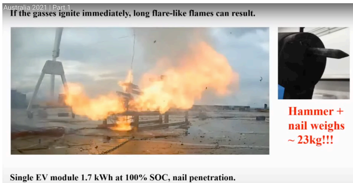
Figure A.3 (f). The “long, flare-like flames” last for several minutes as the fire progresses after the initial explosion and ignition
